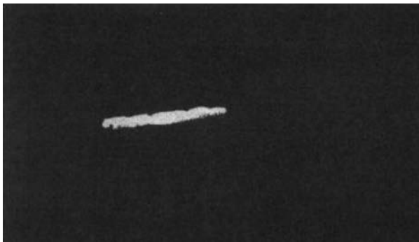
Figure 6 – Track produced by an \alpha – particle
