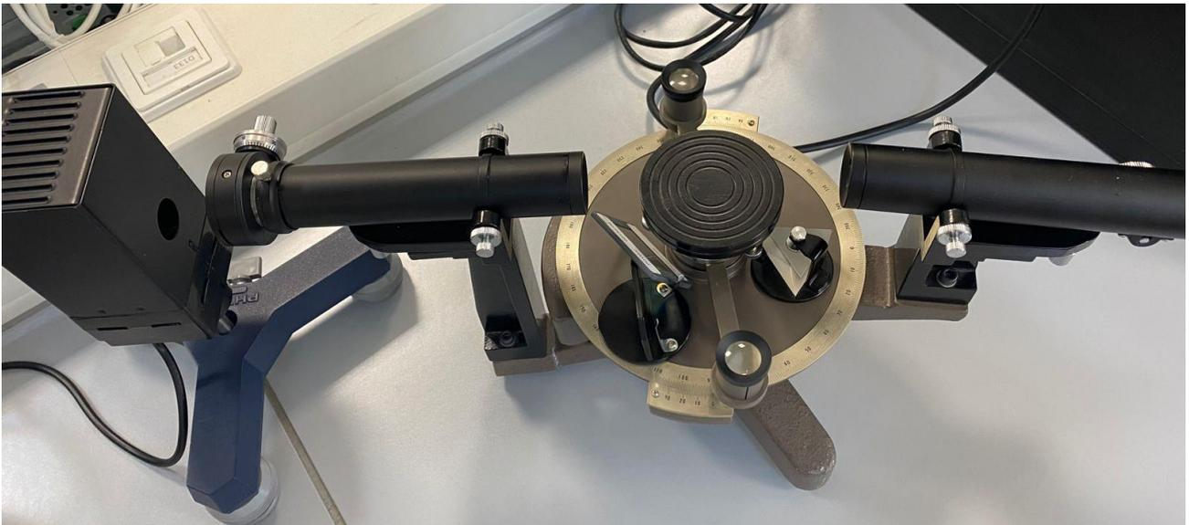
Figure 1 – The instrumental setup of optical spectrometer
