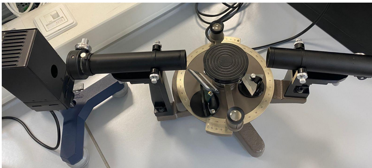
Figure 1 – The instrumental setup of optical spectrometer
